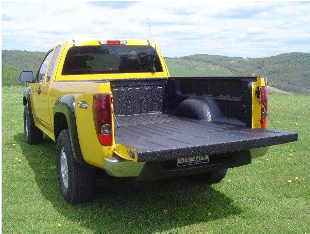
Figure 01: Truck bed liner using permanent ArmorThane polyurethane spray-on protective coating
